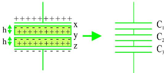
$$\frac{1}{C_{eq}} = \frac{1}{C_1} + \frac{1}{C_2} + \frac{1}{C_3} = \frac{x}{\epsilon_0 A} + \frac{y}{\epsilon_0 A} + \frac{z}{\epsilon_0 A}, x + y + z = 3h$$
